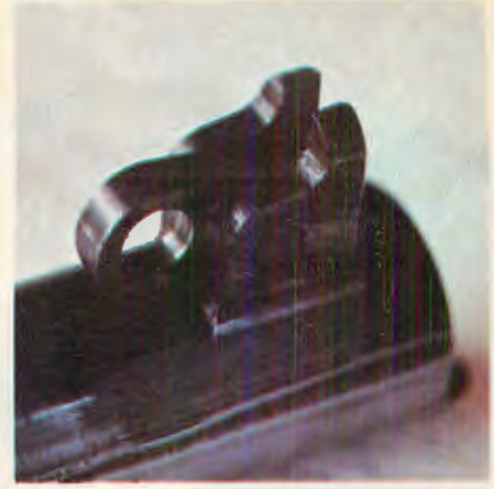
Left: Standard Colt's barrel, showing lugs on underside that push locking cams into recesses inside slide.
